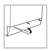
1. using a screwdriver, remove the cover panel on the lower front part of the washer-dryer (see figure);
